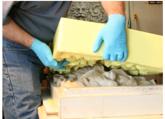
A mold was produced from the restored original piece.
